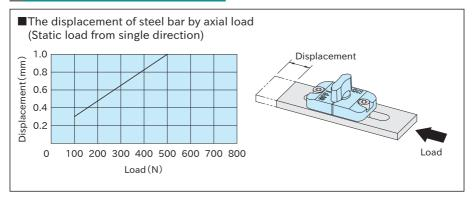
Note: The above data is for a flat bar made of SUS304 stainless steel, SS400 steel and S45C steel. Using an aluminum flat bar, the surface will be scratched or dent by applied load.
