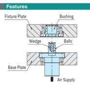
Supply air for unclamping. The wedge goes up and releases the balls.
